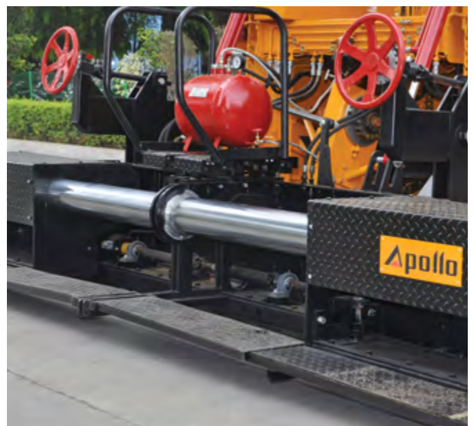
Hydraulically extendable screed.
