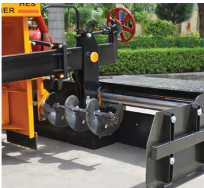
Large diameter augur.
