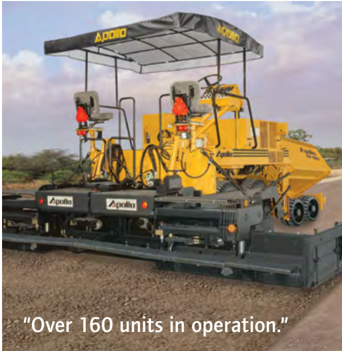
Hydrostatic Sensor Paver Finisher AP 600 on Wet Mix Paving.
