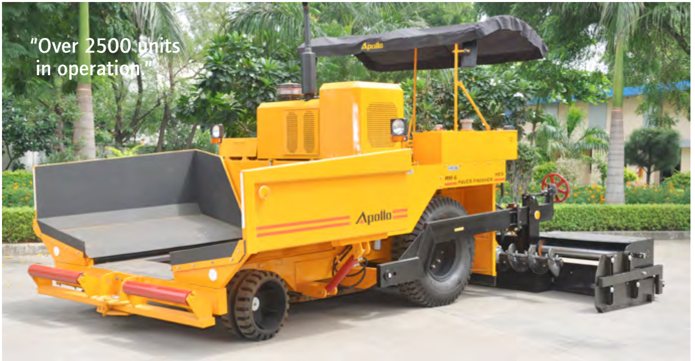
Mechanical Paver Finisher RM 6 HES.
