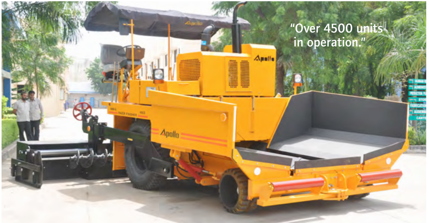
Mechanical Paver Finisher WM 6 HES.
